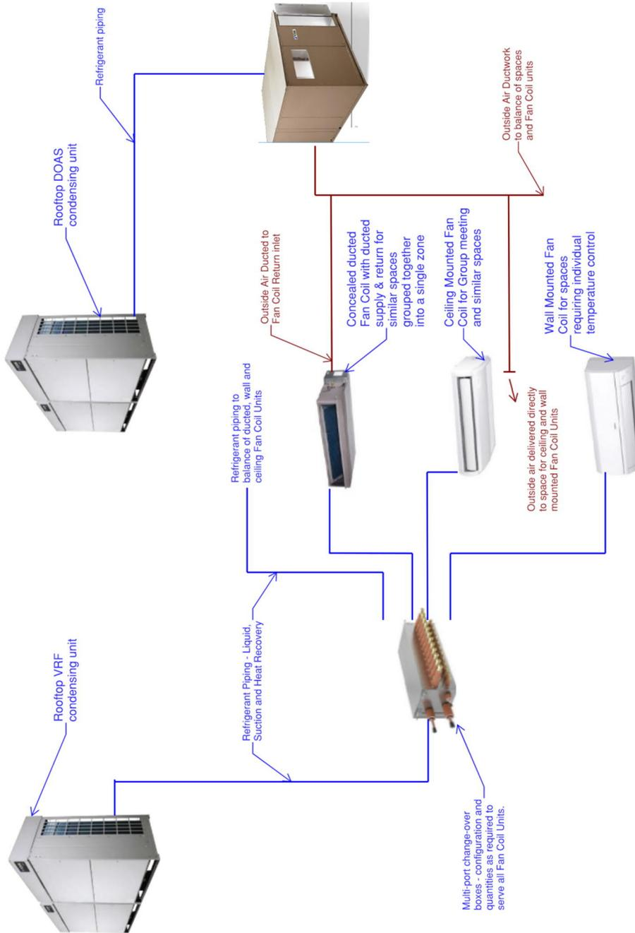
**General Variable Flow Refrigerant & Outside Air System Diagram**
